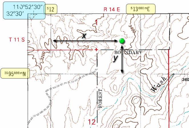
The UTM coordinates in this upper-left corner of a topographic map are highlighted in yellow. The UTM coordinates of the green dot would be easting 512000+x, northing 3595000+y. The numbers highlighted in blue are this map's latitude and longitude at its upper-left corner. Township and range markings are in red.
