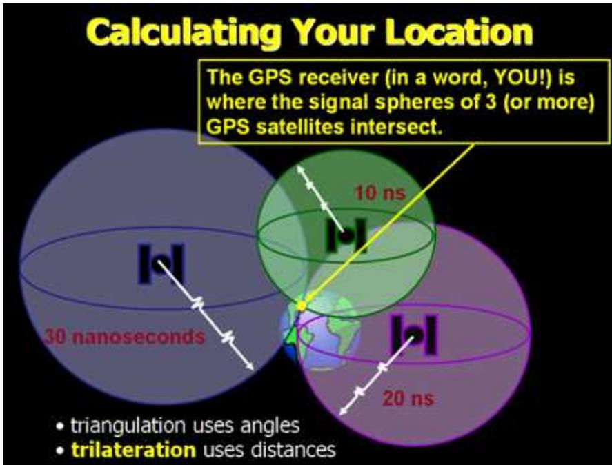
Thus, the GPS receiver measures signal transmission time, which is converted into distance by the above equation. The intersection of the radio signal distances of at least three satellites are used to compute GPS receiver location. This calculation – called *trilateration* – uses the laws of trigonometry, and is conceptually similar to triangulation, but uses distances instead of angles.
