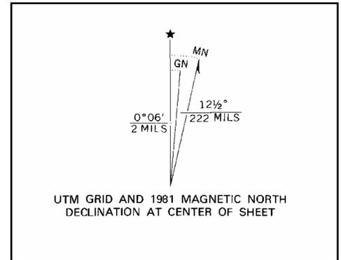
Rather than adding or subtracting each time you take a bearing, you can calibrate most compasses to account for the declination angle by turning a tiny metal screw on the compass housing. For Tucson, Arizona (in May 2004), you would turn the screw to rotate the compass housing so the magnetic north/compass needle mark sits 11.4 degrees to the right (east) of the true north orienting meridian lines.
